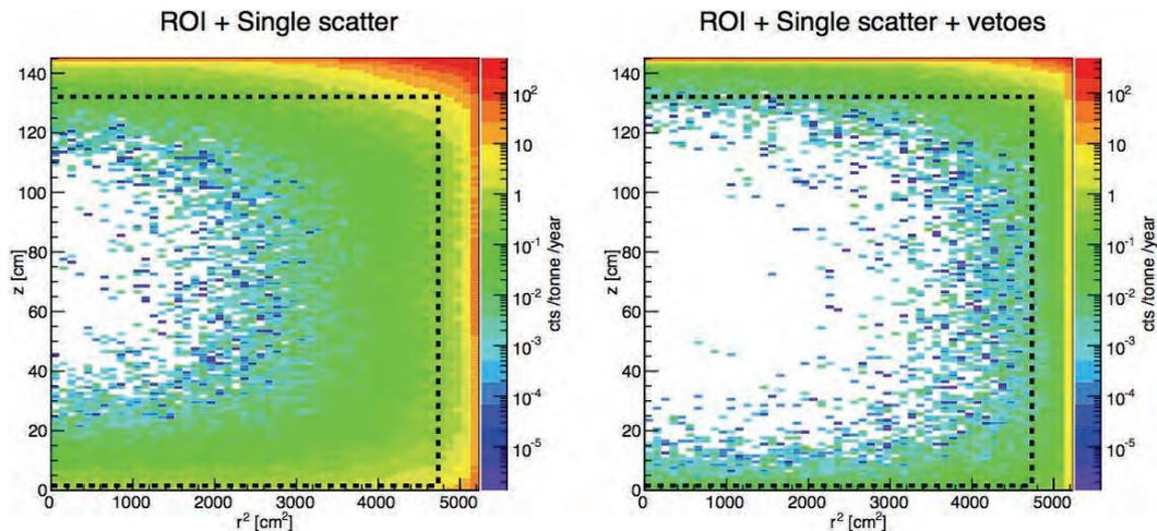
Simulated neutron background in LZ before and after application of veto cuts
