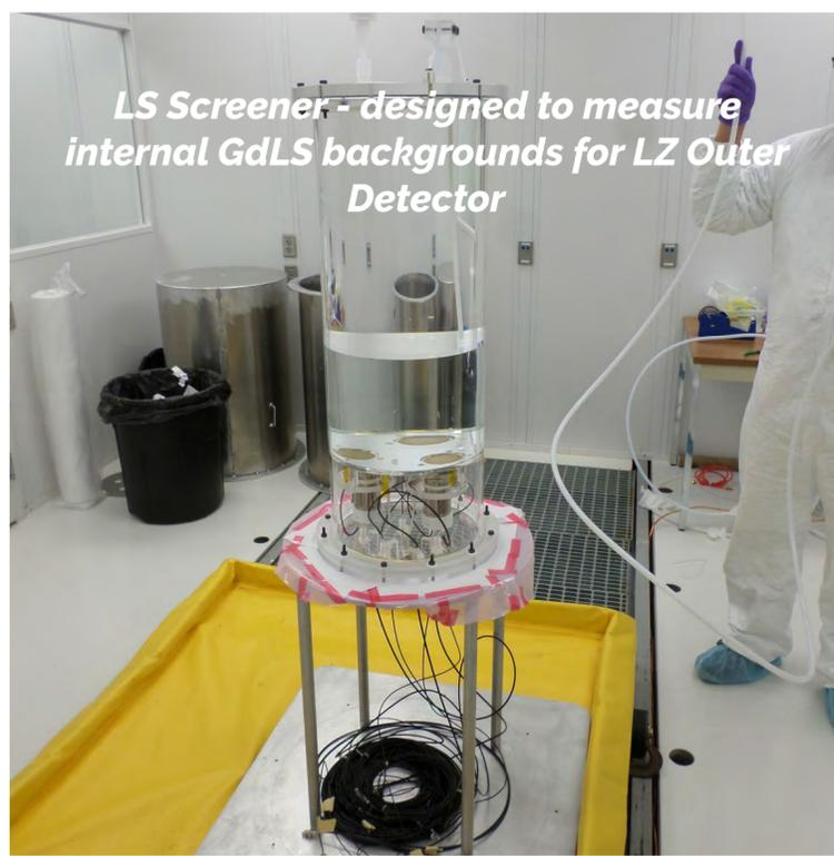
LS Screener - designed to measure internal GdLS backgrounds for LZ Outer Detector
