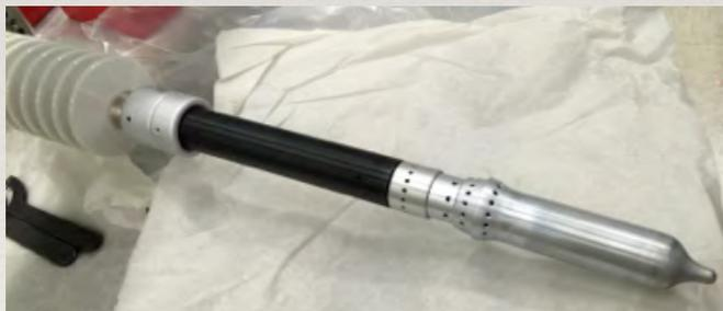
Cathode HV feedthrough
