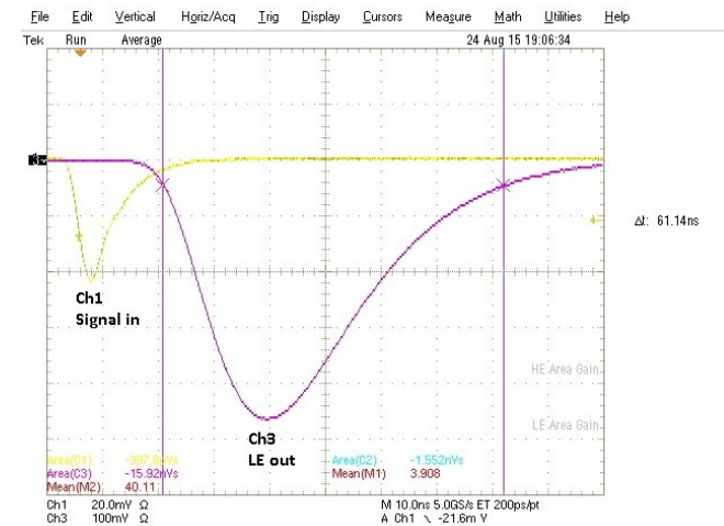
Low-energy channel output with shaping time of 60ns
