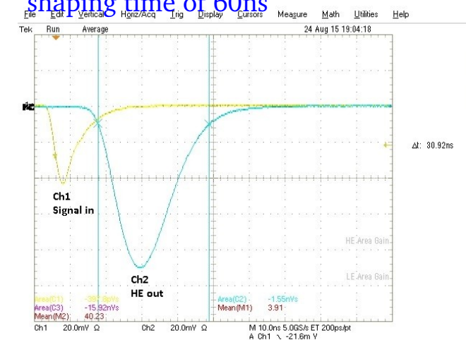
High-energy channel output with shaping time of 30ns
