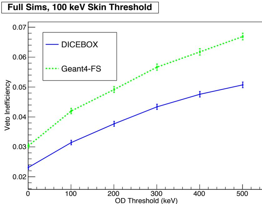
The LZ OD neutron inefficiency vs energy threshold.
