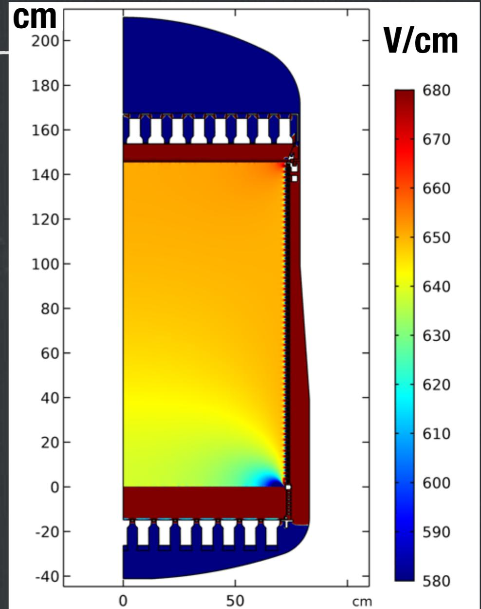
Electric fields in the LZ detector with the cathode at -100 kV
