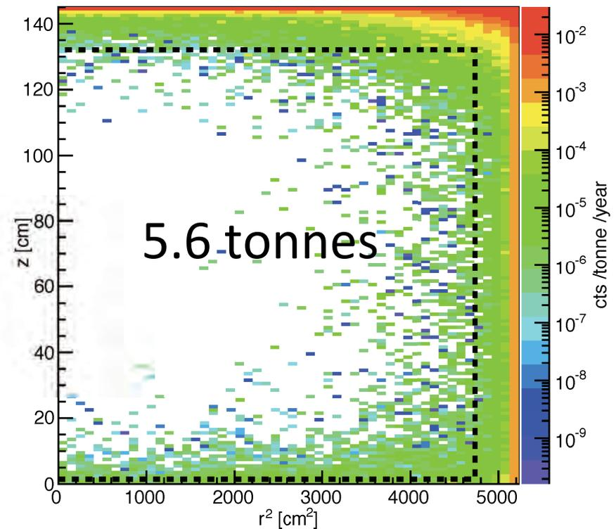
NR background plus ER leakage from sources external to the LXe (6 - 30 keVnr acceptance; 50% NR acceptance and 99.5% ER discrimination);
