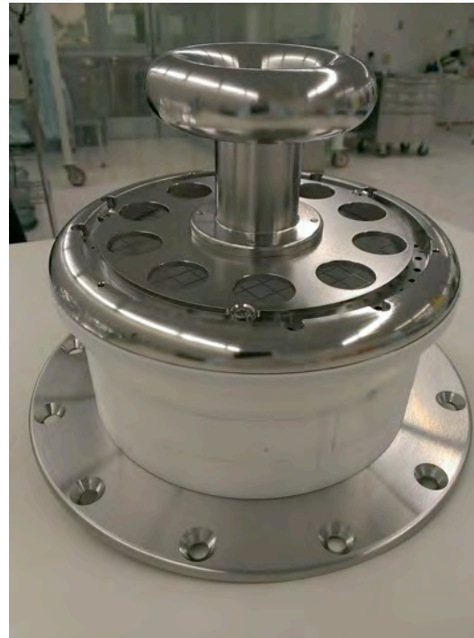
Prototype of highest E-field region tested in LAr
