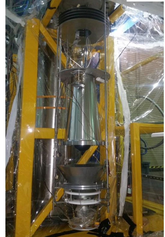
Liquid argon cathode high voltage test facility at LBNL
