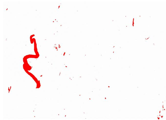
witness coupons image under microscope showing dust particulates of different sizes
