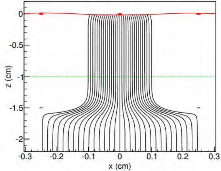
Electron drift lines for gate (-3.5kV, 5mm pitch) and anode (+4kV, 2.5mm pitch) aligned.
