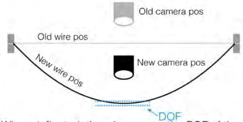
When deflected, the wire causes the POF of the camera to move downward.
