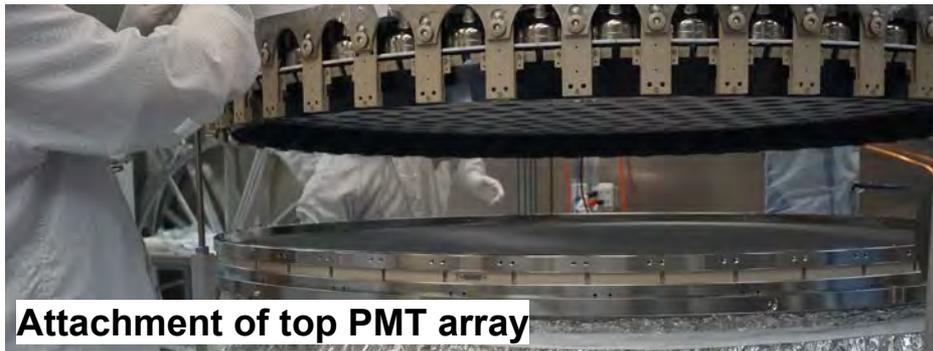
Attachment of top PMT array
