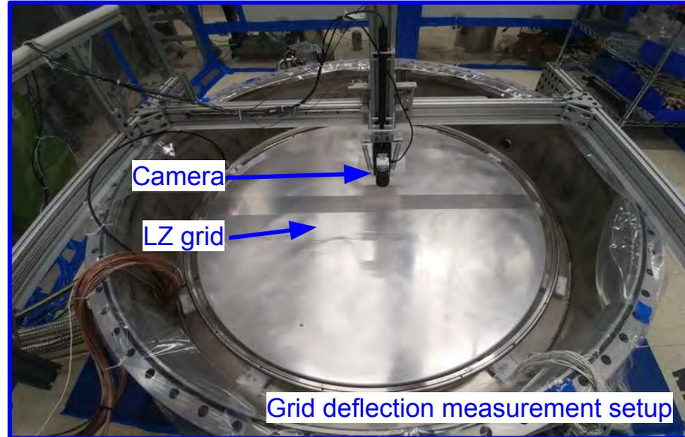
Gate/anode wire alignment mapped for entire extraction region
