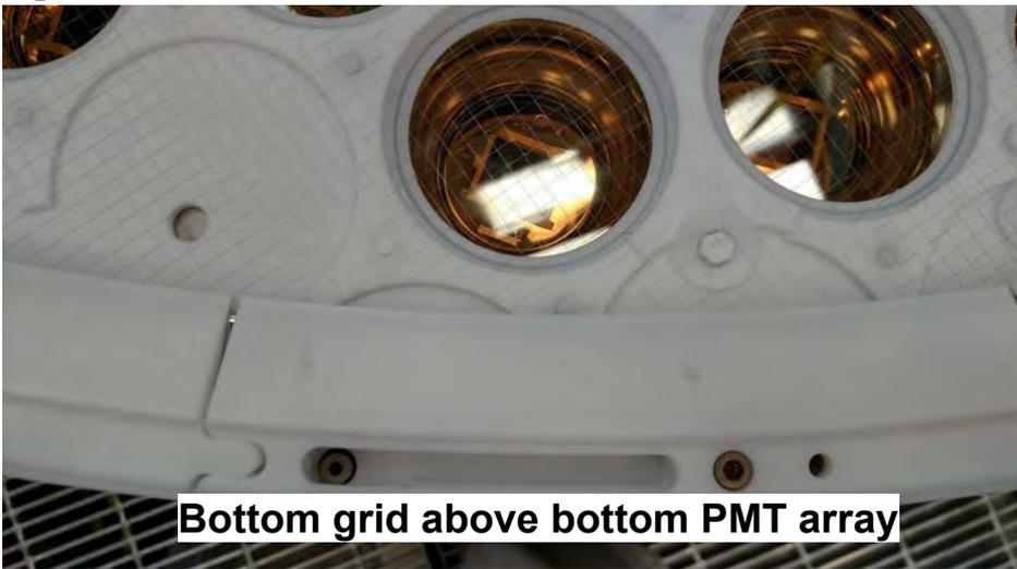
Bottom grid above bottom PMT array
