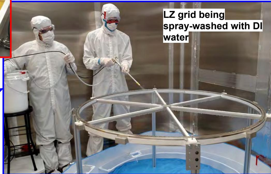
Wash grids with DI water spray prior to installation
