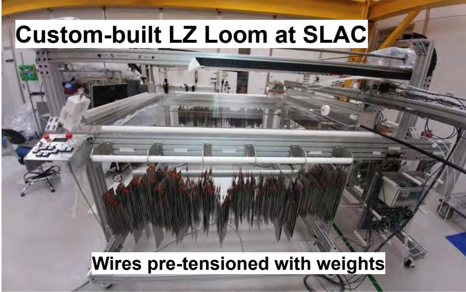
**Wires pre-tensioned with weights**
