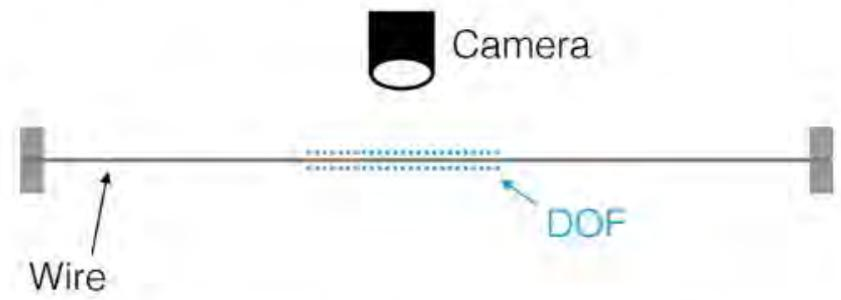
When undeflected, the wire is near the POF of the camera at its original height.
