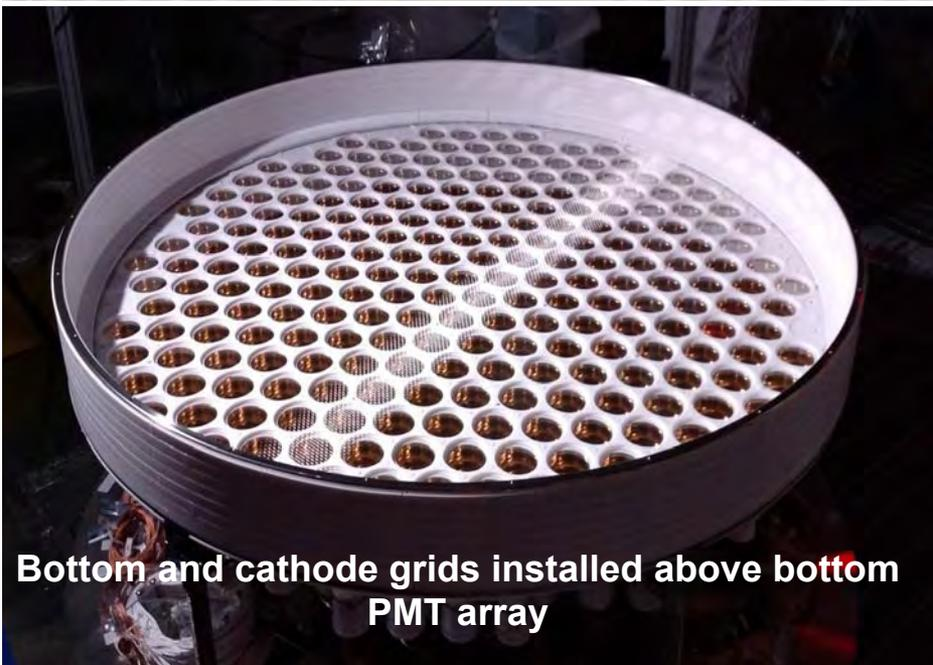
Bottom and cathode grids installed above bottom PMT array
