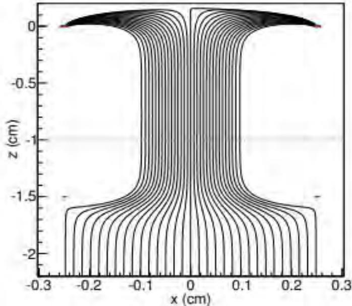
Electron drift lines for gate (-3.5kV) and anode (+4kV) aligned, 5mm pitch. The green line indicates the liquid surface. The red circles and lines are the locations of the wires in the  $y = 0$  plane.
