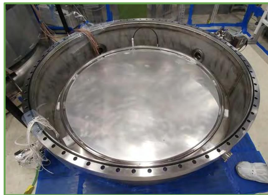
**Full-scale LZ prototype grid installed in vessel**
