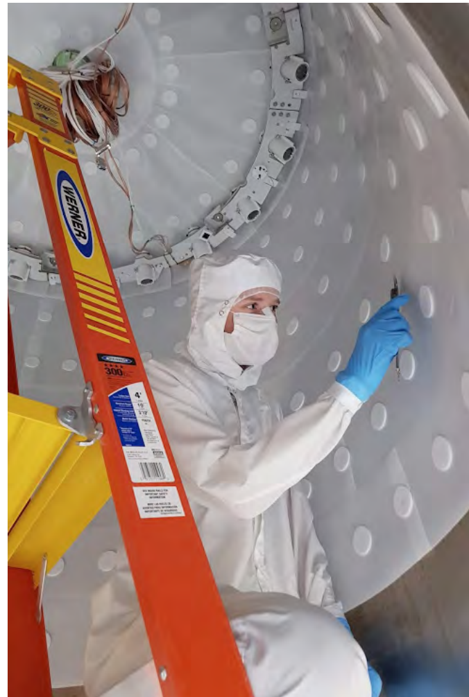
PTFE tiling in ICV & Bottom side skin assembly
